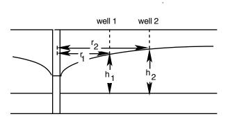
Since h and  $\ln r$  have a straight-line relation, we can substitute  $h_1$  and  $h_2$  for h and  $h_w$ , and  $r_1$  and  $r_2$  for r and  $r_w$ . That is:
