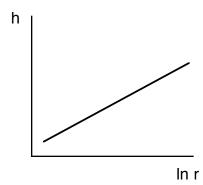
Pumping Test to Determine K
